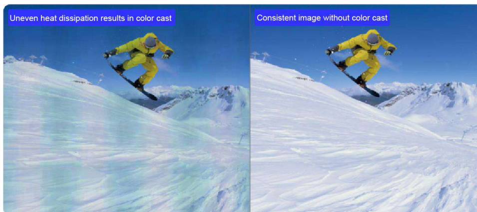
Figure 3-9 Before and after thermal compensation
