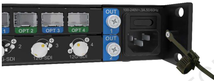
Figure 3-5 Cable clip and cable tie installation
