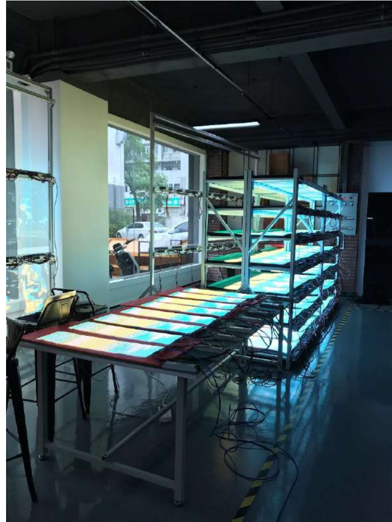
产品7x24小时老化测试 Product 7x24 hours aging test
