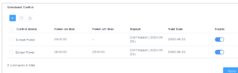
Figure 5-14 Scheduled screen power control
